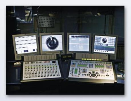
At the heart of the system is the Station Plus Controller with main meter bridge and fader sidecar harnessing the power of a dual card QDC DSP engine. We have added a Pyxis Non Liner Video system, a suite of plug-ins and Medialink networking to allow the seamless integration of this system into a wider networked facility.
